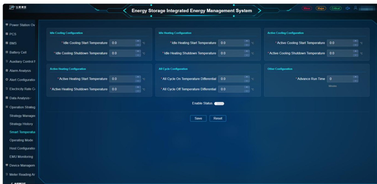
Figure 3-17 Smart Temperature Control
