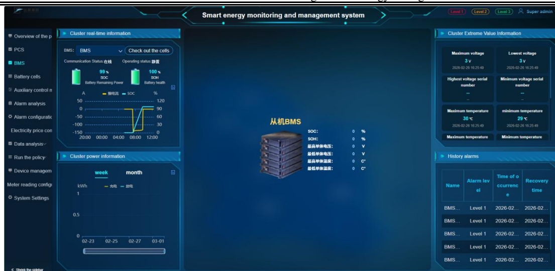
Figure 3-3 BMS Main Interface
