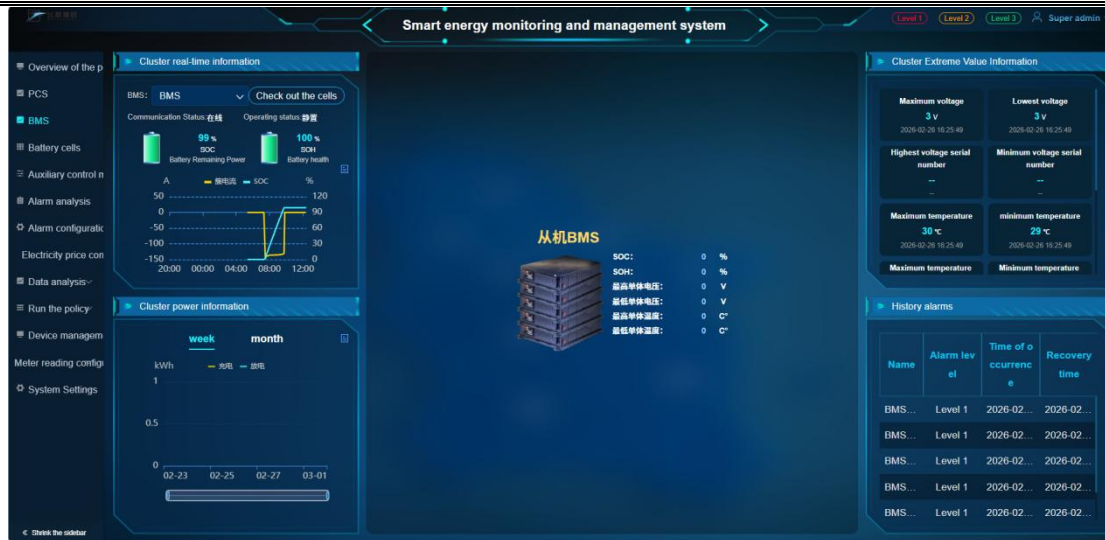
Figure 3-3 BMS Main Interface
